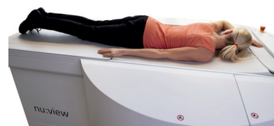
Figure 1. The nu:view Mamma-CT system was developed and is produced by the German company AB-CT - Advanced Breast CT. The design of the new scanner allows compression-free imaging of one breast at a time. To do this, the breast CT system uses a rotating gantry on which the X-ray tube and photon-counting detector are mounted. During the image acquisition process, the gantry rotates around the breast in a downwards-oriented spiral trajectory. In the course of a single scan up to 12,000 projection images are acquired. A full spiral scan takes as little as 7 - 12 seconds. The radiation dose is similar to that of conventional mammography.
